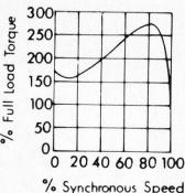
**Design A** covers a wide variety of motors similar to Design B except that their breakdown torque and starting current are higher.
