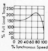
**Design B Motors** are the standard general purpose design. They have low starting current-normal torque, and normal slip. Their field of application is very broad and includes fans, blowers, pumps, and machine tools. Torque values are listed in this Modification Section.
