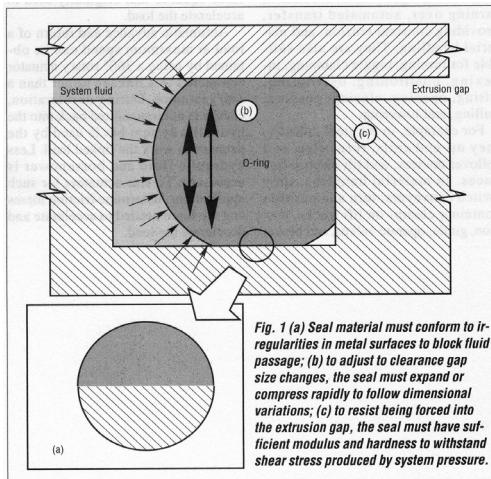
Fig. 1 (a) Seal material must conform to irregularities in metal surfaces to block fluid passage; (b) to adjust to clearance gap size changes, the seal must expand or compress rapidly to follow dimensional variations; (c) to resist being forced into the extrusion gap, the seal must have sufficient modulus and hardness to withstand shear stress produced by system pressure.
