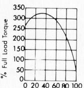
**Design D Motors** have a high breakaway torque combined with high slip. Breakaway torque for 4,6 and 8 pole motors is 275% or more of full load torque. Two slip groups are described below.
