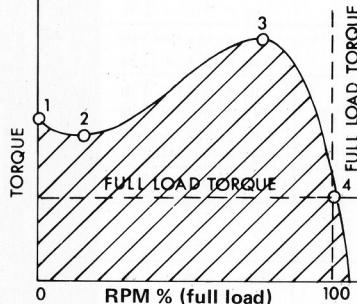
The sectioned area under the curve represents a motor's accelerating torque from zero to full speed. Torque, horsepower, and speed requirements demanded in drives for most machines can be met with one of four design classes of squirrel-cage polyphase induction motors described by National Electrical Manufacturers Association standards.
