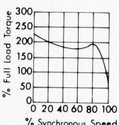
**Design C Motors** have high breakaway torque, low starting current, and normal slip. The higher breakaway torque makes this motor advantageous for "hard-to-start" applications, such as plunger pumps, conveyors, and compressors.
