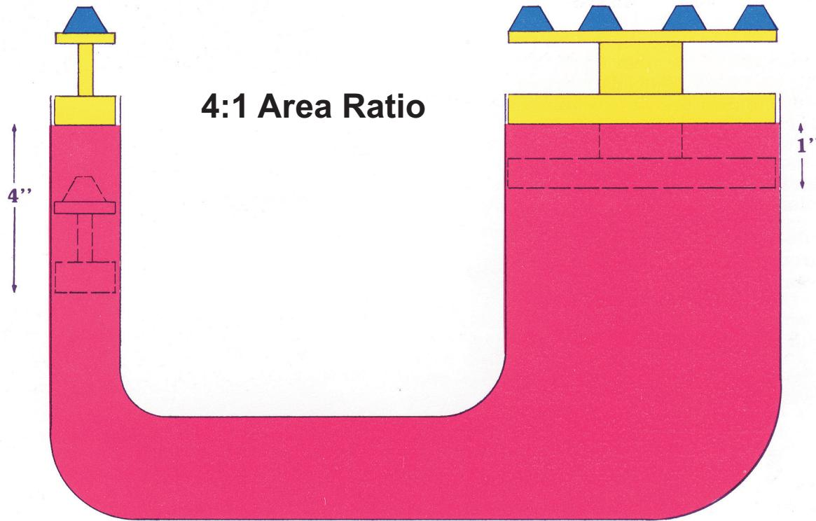
We gain a force advantage (multiplier) at the cost of stroke (distance). This is always the 'area ratio'.
